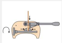
Insert large diameter mandrel followed by the coated test panel, making sure that the painted area faces away from the mandrel.
