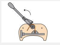
With a smooth action pull the lever around the mandrel. Check coating for damage.
